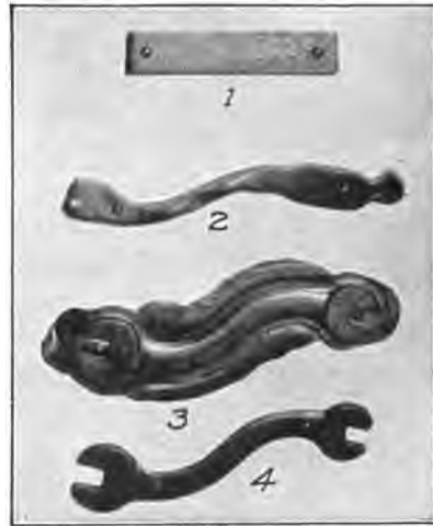
Fig. 172. Steps in Forging S-Wrench
